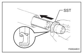
(d) Install the "Teflon" ring into the steering rack's groove. Grip the ring to press it into the groove.
