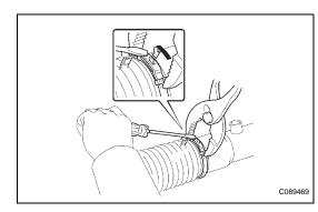
(d) Using SST, install the power steering rack end (LH side) onto the power steering rack.
