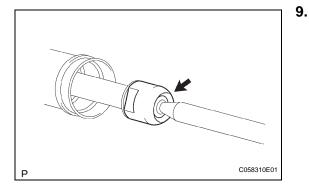
Using a 24 mm hexagon wrench, hold the rack guide spring cap. Using SST, torque the nut.
